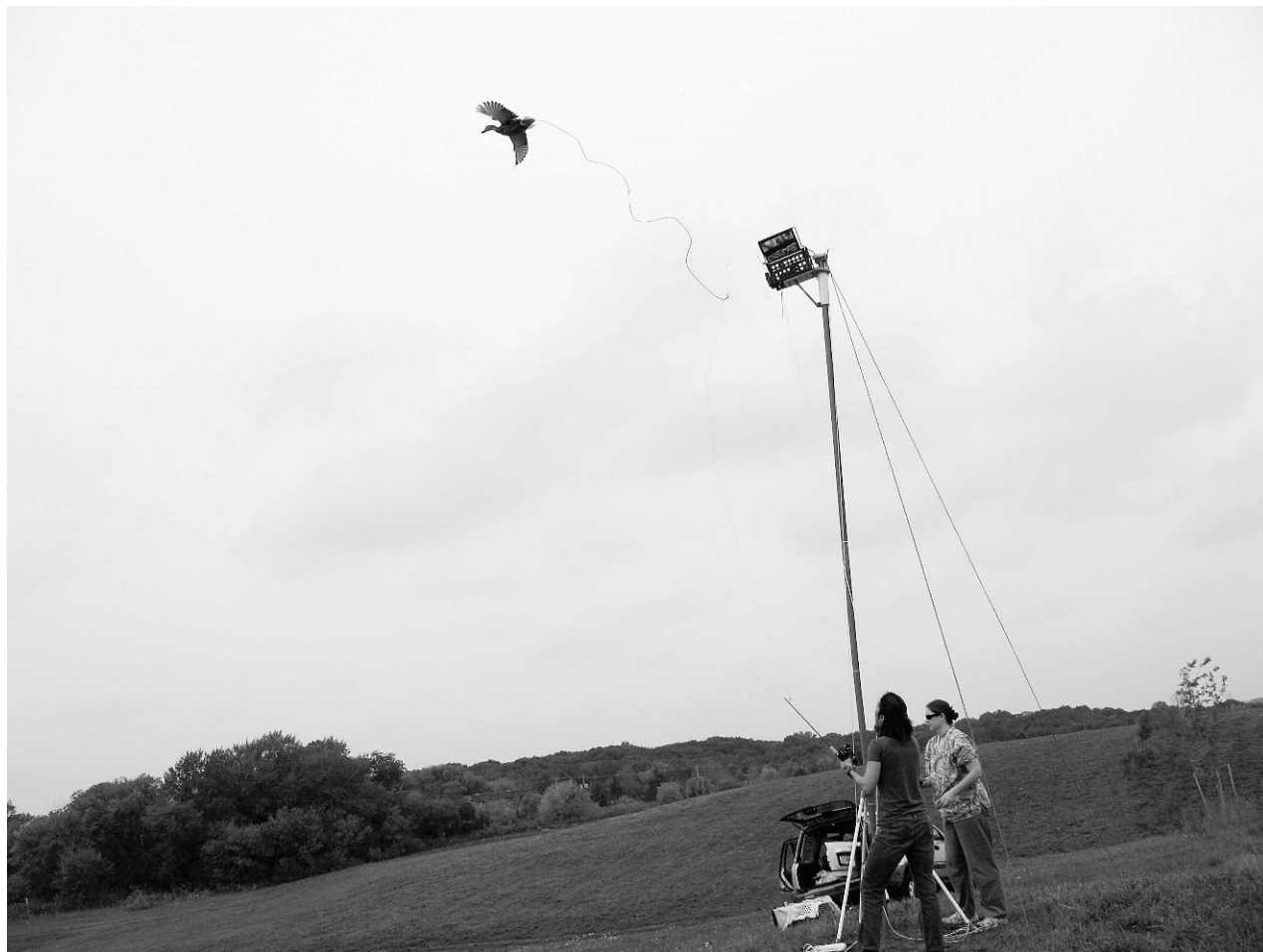
Figure 2. The study mallard is launched from the portable tower and remote-controlled launcher for a conditioning flight.
